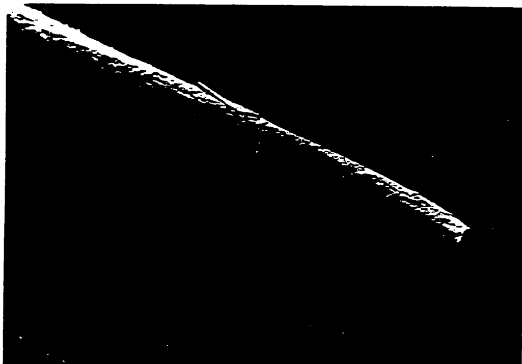
Figure 6.2.8. Untreated 5 \mu\text{m} silver wire ( 200 times magnification ).
