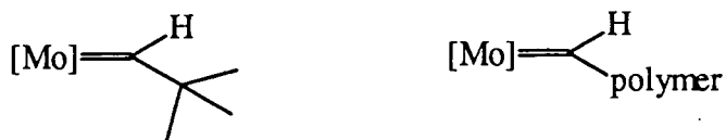
Figure 3.16 Initiating (left) and propagating (right) alkylidene hydrogens. Molybdenum and its associated ligands are represented as [Mo].
