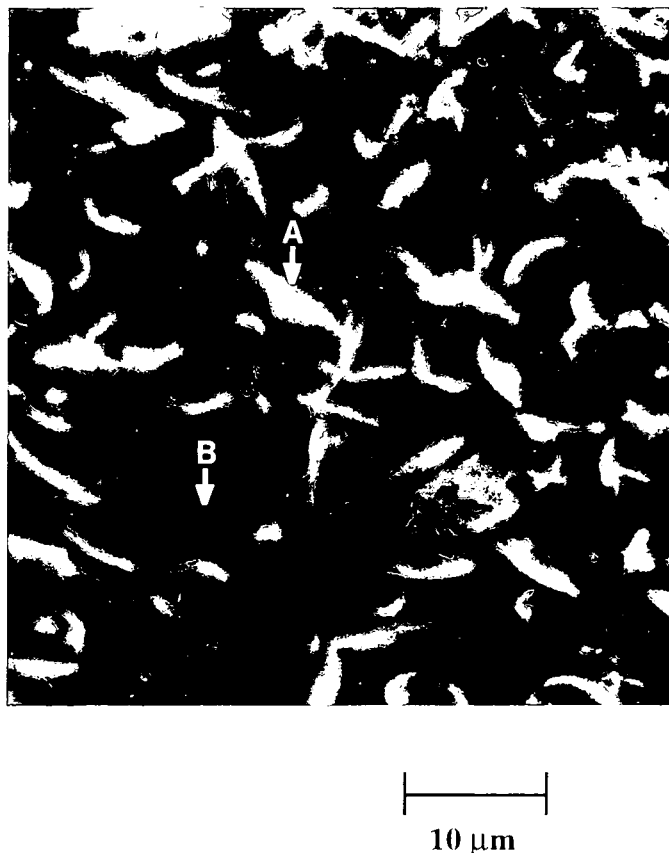
Fig. 6.17 Scanning electron micrograph of an iodine doped 79-layer film of OA:ODTTF in the ratio 1:2.3. The sample was coated with silver to prevent charging by the electron probe.
