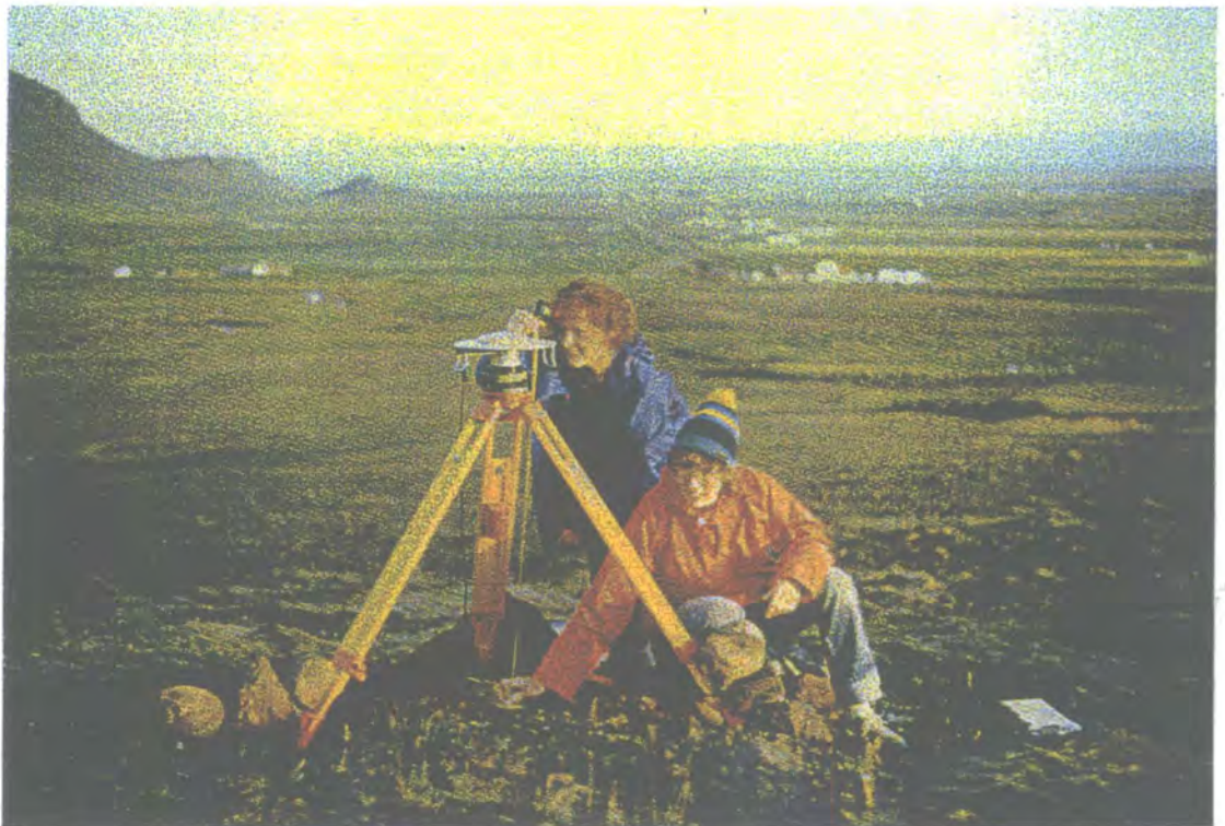
Figure 3.4. Photograph showing the typical field set-up for a GPS receiver to determine accurate locations of each station in the temporary array.
