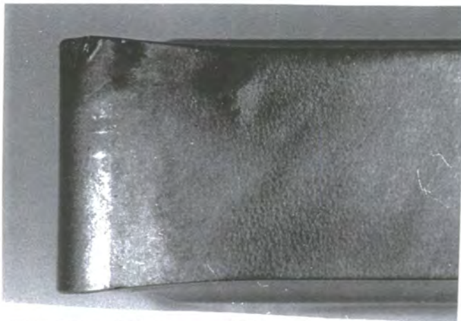
Test 4 ( a = 1.6 mm, s = 0.28 mm/rev, v = 295 m/min)
