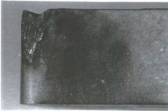
Test 3 ( a = 1.7 mm, s = 0.25 mm/rev, v = 310 m/min)
