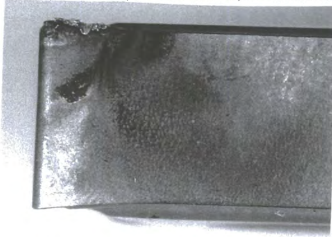
Test 3 ( a = 1.4 \text{ mm} , s = 0.17 \text{ mm/rev} , v = 360 \text{ m/min} )
