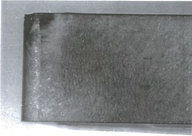
Test 2 ( a = 1.1 \text{ mm} , s = 0.19 \text{ mm/rev} , v = 390 \text{ m/min} )
