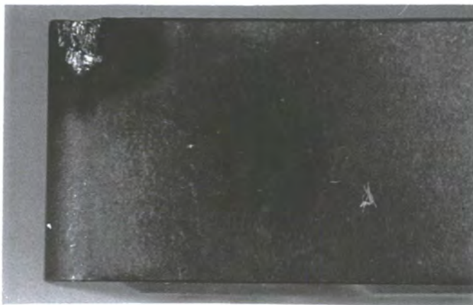
Test 3 ( a = 1.0 \text{ mm} , s = 0.2 \text{ mm/rev} , v = 400 \text{ m/min} )
