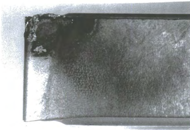
Test 5 ( a = 1.5 \text{ mm} , s = 0.18 \text{ mm/rev} , v = 430 \text{ m/min} )
