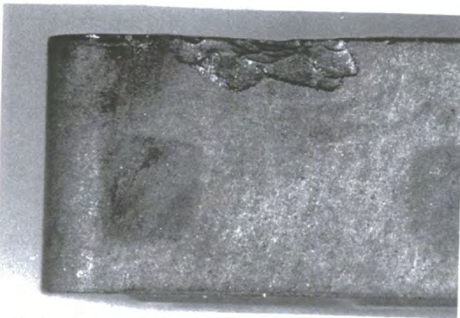
Test 4 ( a = 0.7 \text{ mm} , s = 0.23 \text{ mm/rev} , v = 450 \text{ m/min} )
