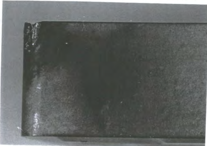
Test 3 ( a = 1.5 \text{ mm} , s = 0.2 \text{ mm/rev} , v = 395 \text{ m/min} )
