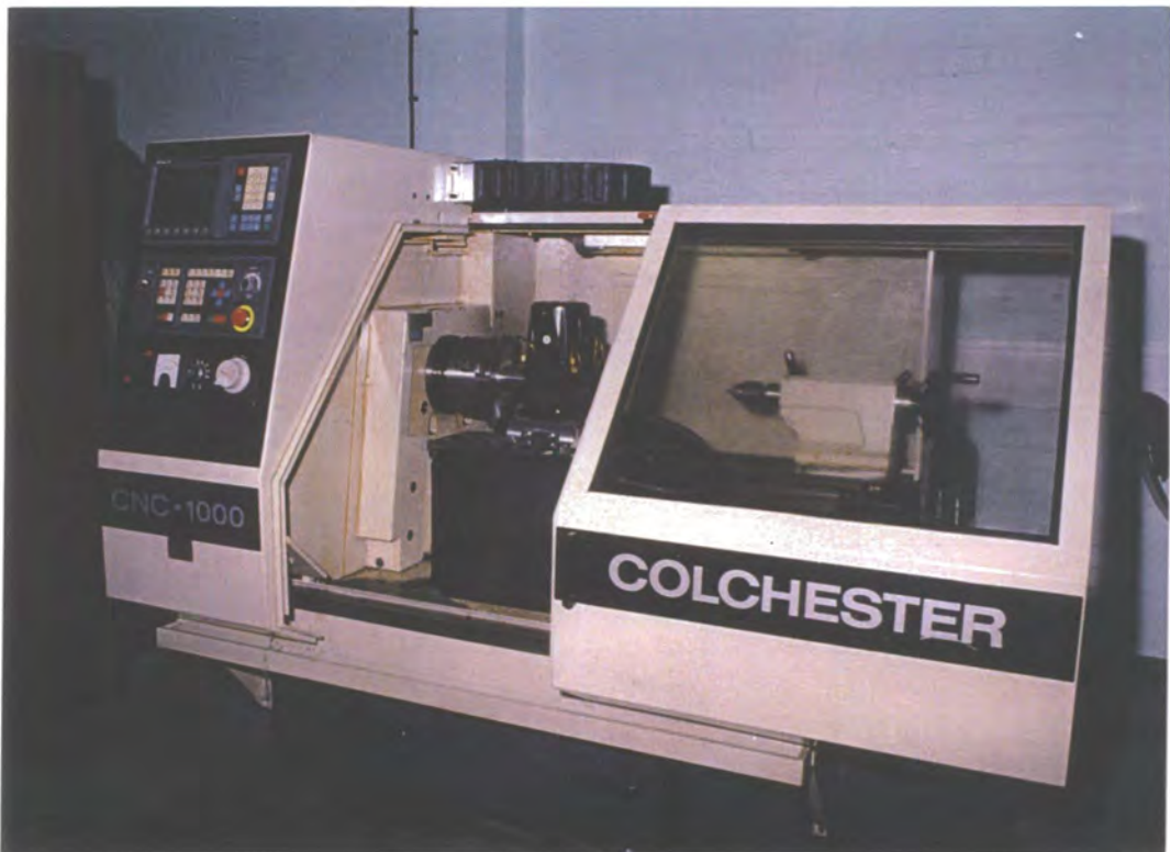
Figure 5.1 Colchester CNC-1000 centre lathe
