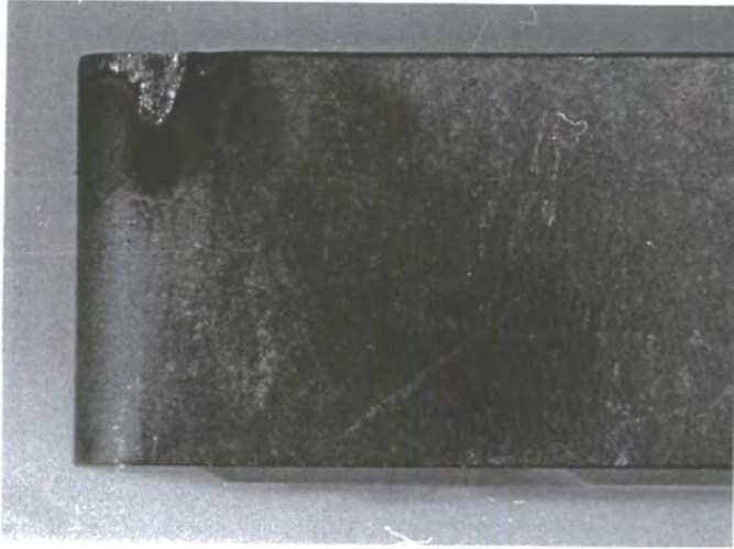
Test 1 ( a = 1.3 \text{ mm} , s = 0.15 \text{ mm/rev} , v = 415 \text{ m/min} )
