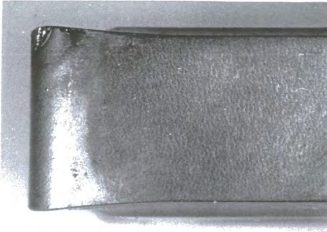
Test 1 ( a = 3.0 mm, s = 0.25 mm/rev, v = 150 m/min)
