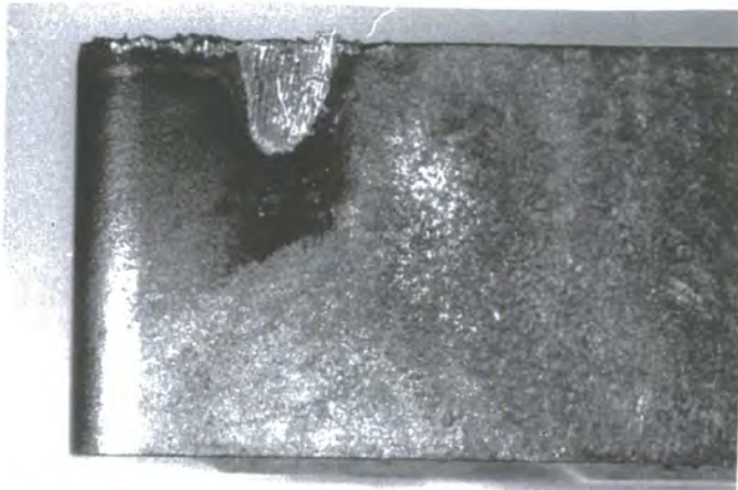
Test 2 ( a = 3.0 mm, s = 0.25 mm/rev, v = 120 m/min)
