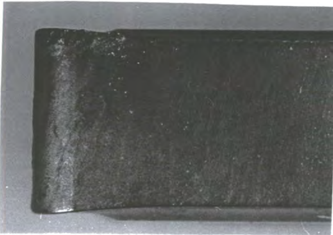
Test 2 ( a = 3.0 mm, s = 0.3 mm/rev, v = 125 m/min)
