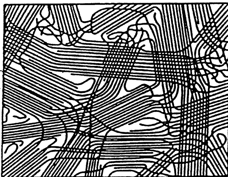
Figure 4.4. Fringed micelle model for a semi-crystalline polymer
