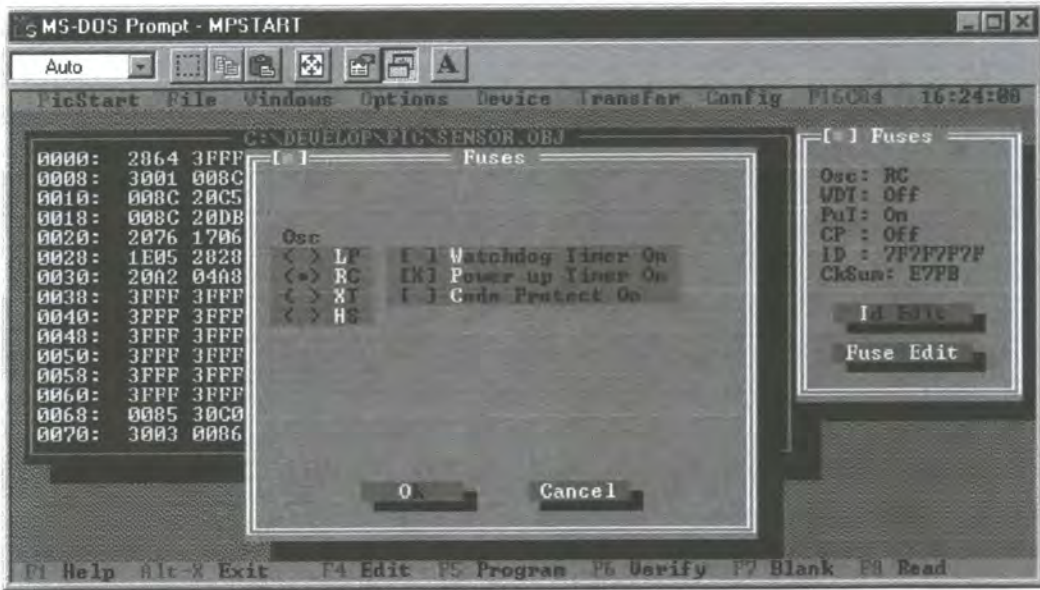
Figure 3.3. The MSDOS software program used to program the PIC processor object code into the device and configure its fuses.
