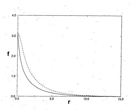
fig. 2.9: The profile function f as a function of r for  $\kappa = \kappa_{cr}^{l} = 0.632$ , N = -1 (solid) and N = -2 (dashed).
