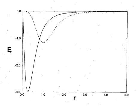
fig. 2.10: The radial component of the magnetic field  $\mathbf{E}_{\mathbf{r}}$  as a function of r for  $\kappa = \kappa_{cr}^{l} = 0.632$ , N = -1 (solid) and N = -2 (dashed).
