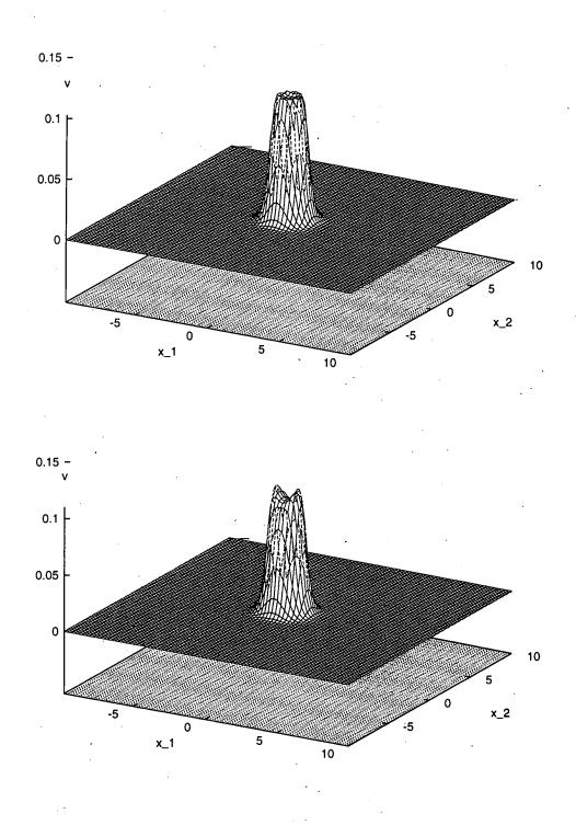
fig. 5.6: Gradient-flow for two-soliton configuration after 2000 timesteps (top) and 12000 timesteps (bottom). The initial values are  $\psi_1 = 0.05$ ,  $\psi_2 = 0$ ,  $\psi_3 = 0.1$ . The couplings are  $\mu_F = 0.1$  and  $\mu_U = 0.01$ .
