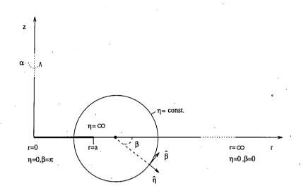
fig. 4.3: Toridal coordinates  $(\eta, \beta, \alpha)$  and their relation to cylindrical coordinates.
