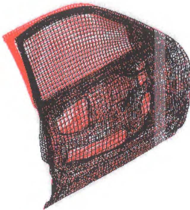
Figure 7-8. Deformation quarter view of model 1 at the 3rd natural frequency
