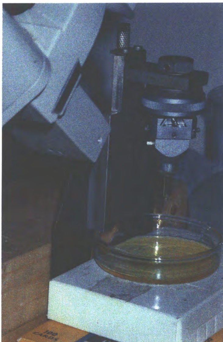
Figure 6.3.1 - The solvent cutting apparatus used to cut the DCNP crystal for the 100K X-ray charge density study.
