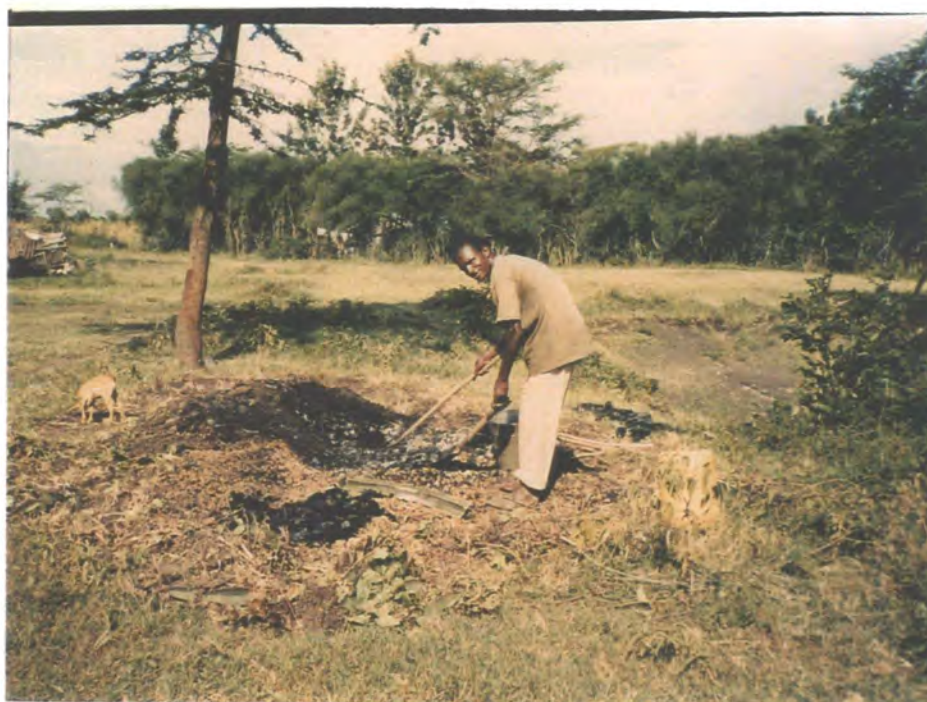
Plate 6.1 (b): Making charcoal 'on site' from branches lopped off an isolated tree above.
