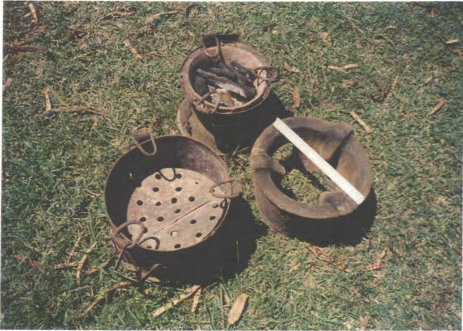
Plate 7.2 (a): An Upesi Jiko (with scale ruler on top) frame without the bottom mounting.
