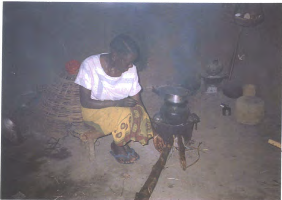
Plate 7.2 (b): An Upesi Jiko being used inside a traditional rural kitchen. Note the characteristic 'two sticks' and small pot.
