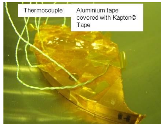
Figure 44: Thermocouple testing in a temperature controlled oven
