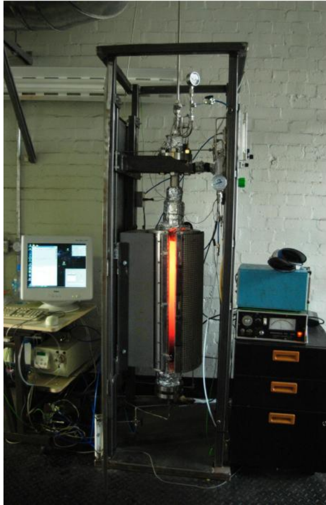
Figure 5.2: Pressurised vessel and the preheating zone of the tests facilities.
