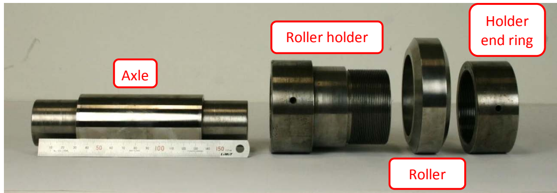
Figure 79: Roller assembly. The roller holder, roller, and end ring rotate together on the axle.
