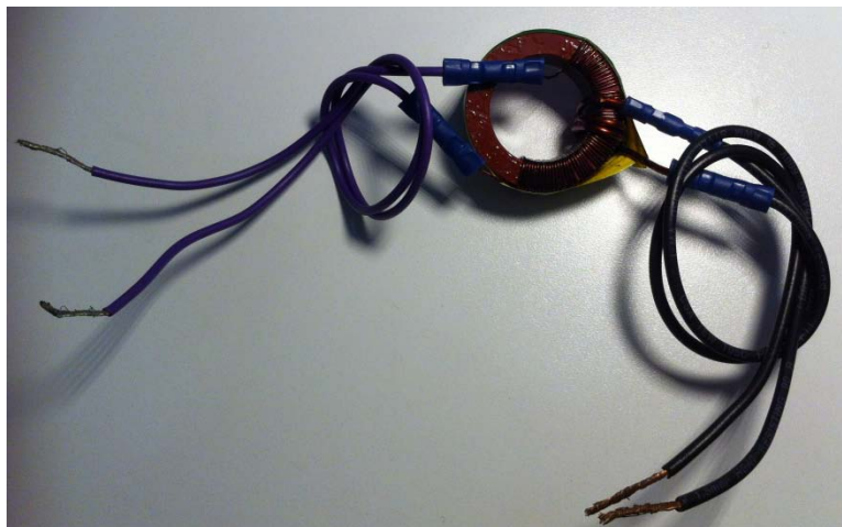
Fig. 3.7: A toroidal amorphous metglas transformer (AMT)
