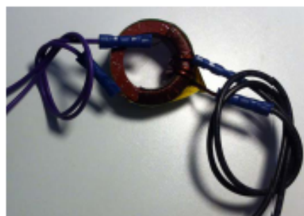
Fig. 6. HF Transformer used in the proposed UPS system
