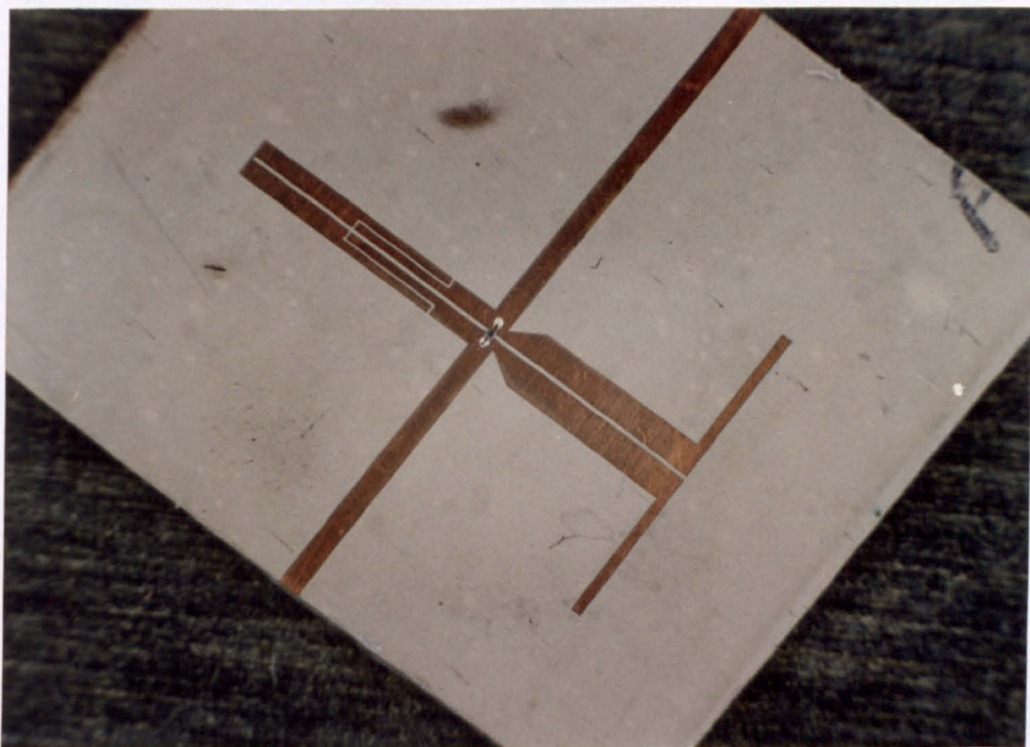
Figure B.4: 10GHz single PIN diode phase shifter with even mode loading. (Magnification: x5.6)
