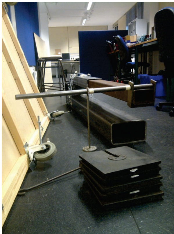
Figure 6-15 Asymmetric load application, 300mm offset from centreline
