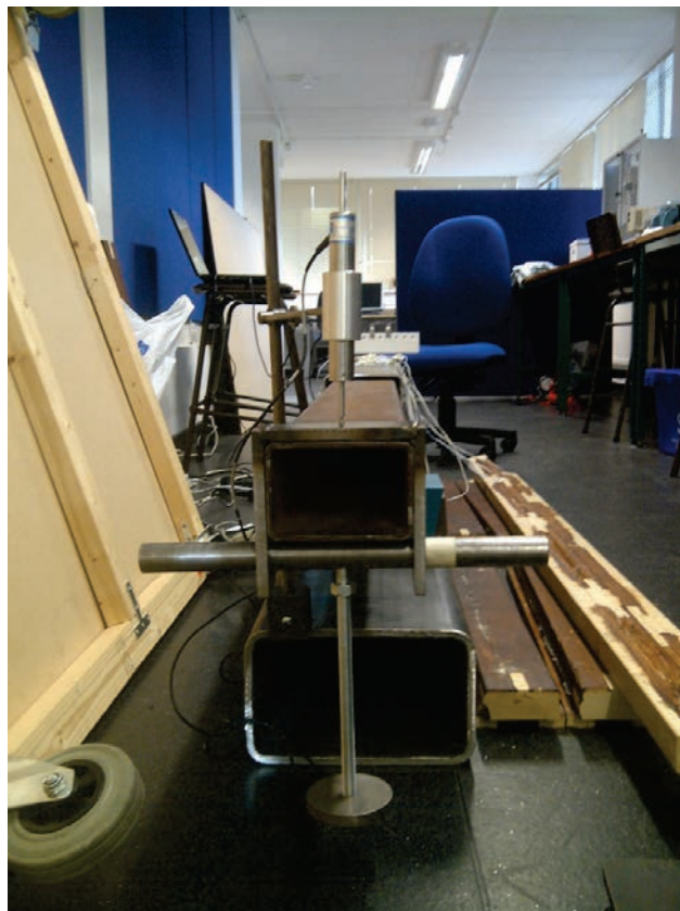
Figure 6-20 Tip displacement experimental measurement with dial gauge
