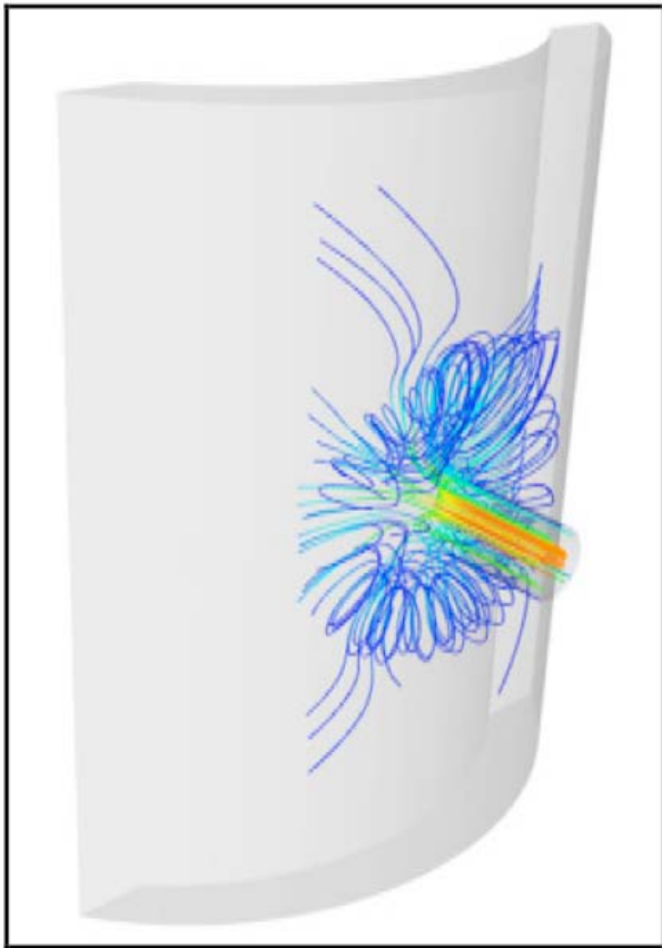
Fig. 10 streamlines of the incoming flow in the vicinity feedhole for flow rate \alpha = 1.0 , \Psi = 10\% and \varepsilon = 0.9 , numerical simulation.
