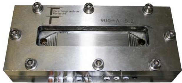
Fig. 5: Electrically powered microstructure device, providing exchangeable micro channel foils and a glass lid for high speed videography.
