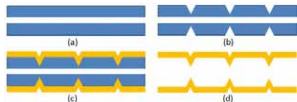
Fig.2 Process steps for the fabrication of rough tubes making (a) Substratum tube (b) Rough structure making on the tube (c) Nickel layer depositing (d) Erasing of substratum
