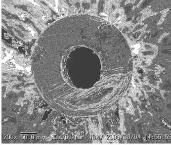
Fig. 3 SEM picture of the micro-tube cross section
