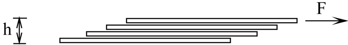
Fig. 2.1. A deck of cards sliding with respect to one another due to the effect of a force F applied at one end.
