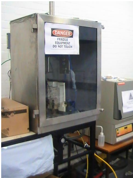
Fig. 3.2. (a) left , actual Couette equipment; (b) right , Schematic representation – Couette type. The bob rod is attached with the torsion wire which is connected to the torque measuring unit on top of a vertical air bearing. The torque measuring unit is connected to the computer which records the raw data. The arrangement is enclosed in a steel cabinet with a glass front door (inset in left picture) which enables evacuation of the chamber and filling with nitrogen gas during experiments at elevated temperatures.
