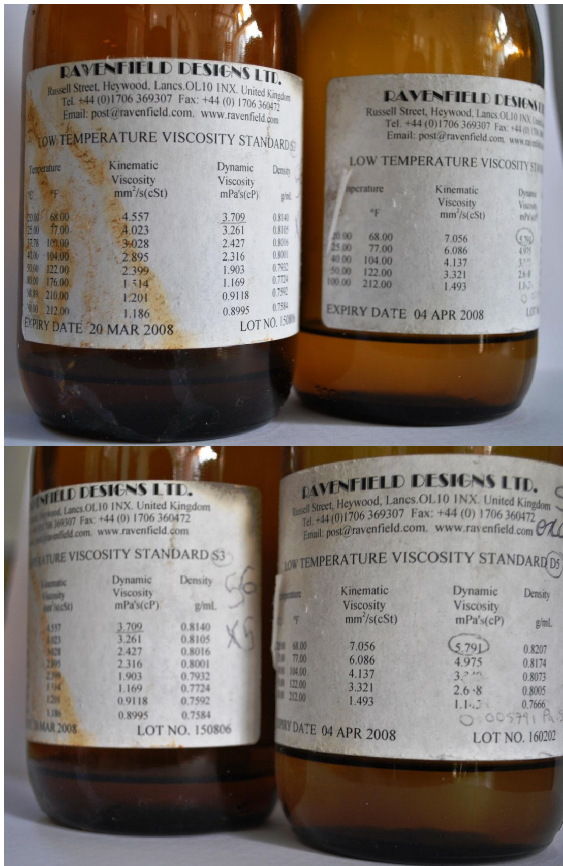
Standard oils employed for calibrating and verifying the Searle type equipment: G3 and D5.
