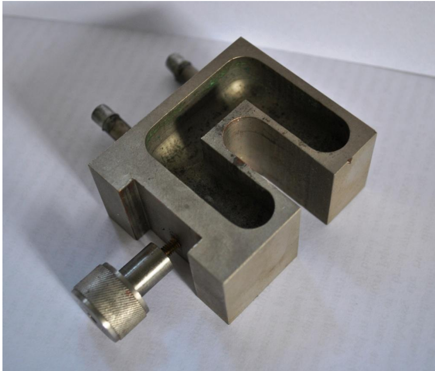
Fig. 3.12. Older version of the chilling unit. The bob-rod had a copper piece which fit in the U-shaped groove, which contained kerosene based oil to provide cooling to the bob.
