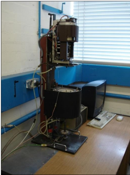
Fig. 3.1. (a) left , Actual Searle equipment; (b) right , Schematic representation – Searle type. The rotating bob rod is connected with the torque measuring unit which is connected to the computer which records the raw data.
