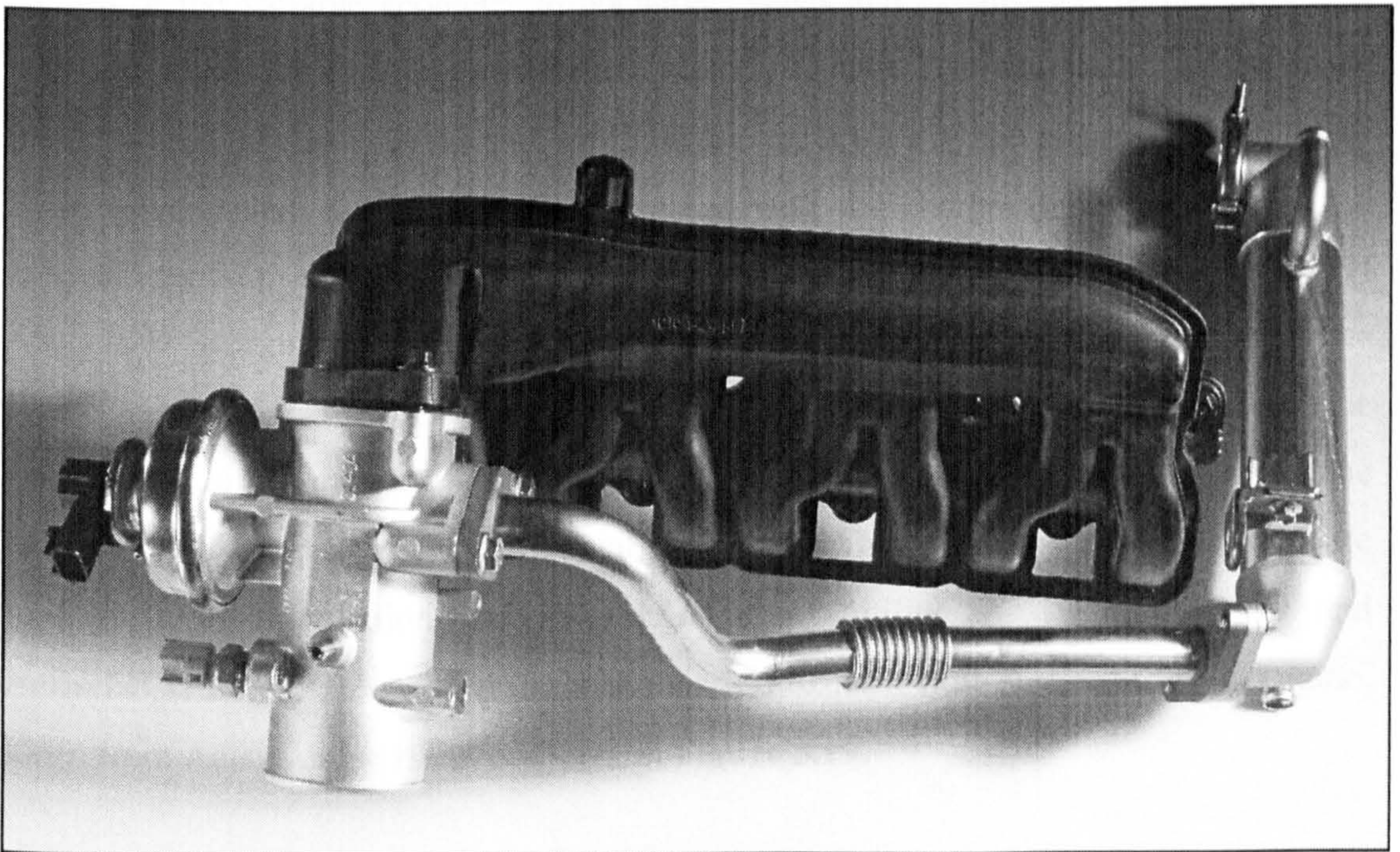
Figures 3.17 and 3.18 Ford DURATORQ diesel EGR System layout and components (Lawrence et al, 1999)
