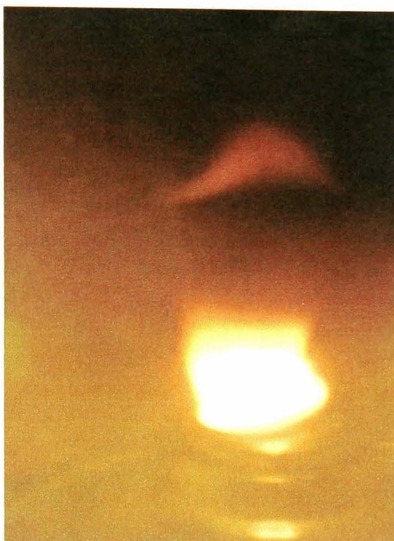
Figure 5-8: The effect of electric field on the shape of a paraffin flame: A) with 5KV applied voltage, B) with 15KV applied voltage
