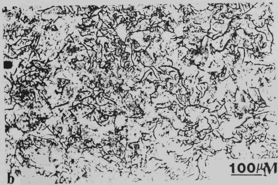
Fig. 29 Microstructure of the liner: a) Unetched b) Etched
