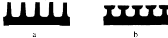
Figure 2.16 Profiles of (a) GEWA – K (b) GEWA – T Ayub and Bergles (1987)
