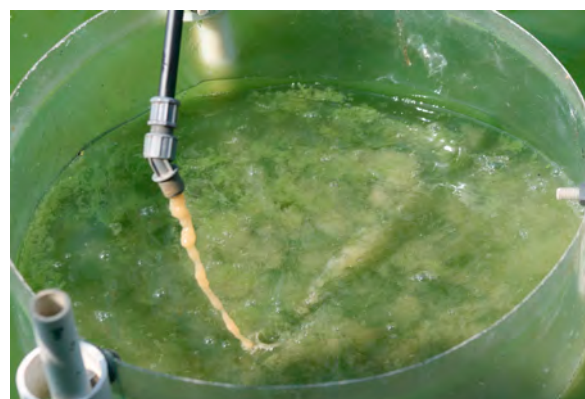
Fig. 1 In situ mesocosm testing of clay flocculation effects on a Microcystis aeruginosa bloom.
