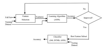
FIGURE 2. Feature selection process: Feature subsets evaluation based on ANN
