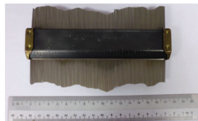
FIGURE 3. Standard 15 cm Barton comb used to reproduce the true roughness profiles of discontinuity surfaces
