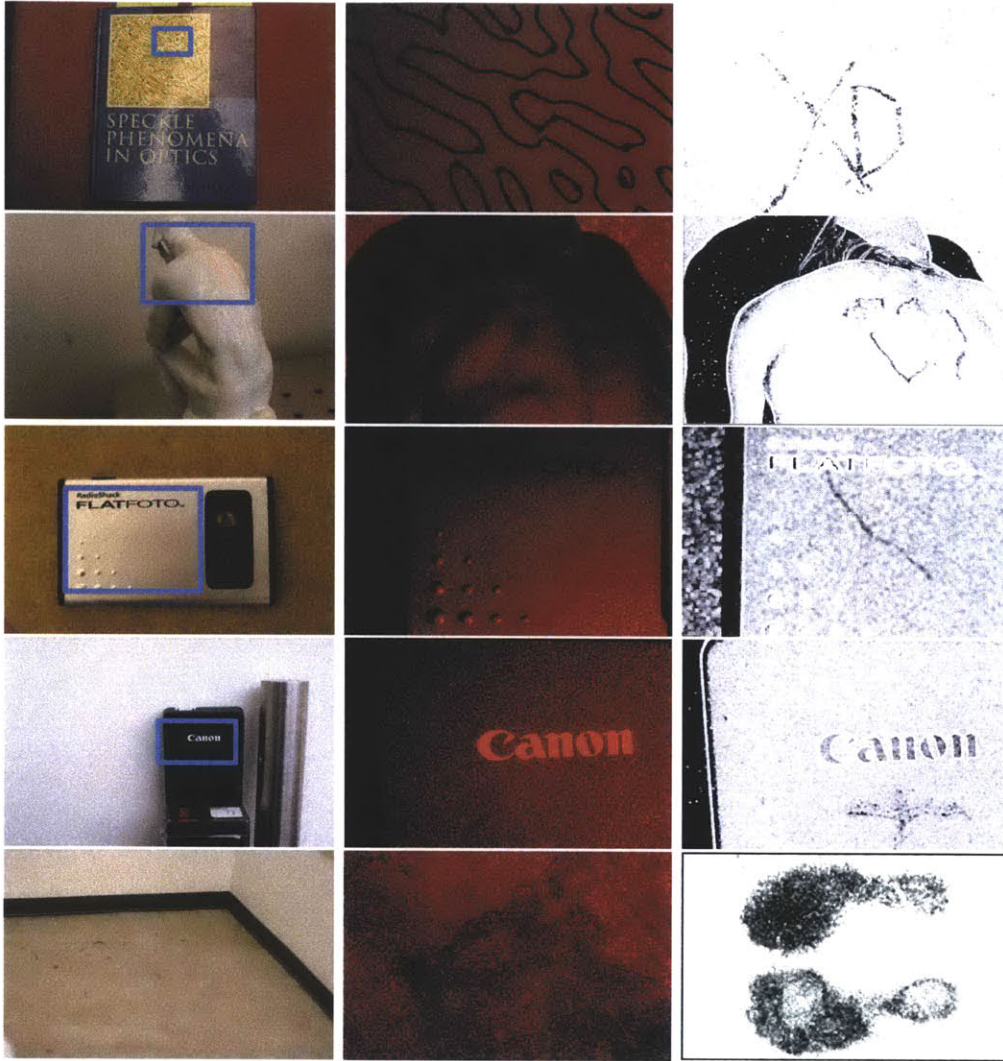
Figure 5-3: Surface tampering detection on different materials using our system. From top to bottom: a glossy textbook cover with a textured design (we drew an XD on it with the fleshy part of a finger), a stone statue (drew a smile), a brushed aluminum camera (drew a backslash), a black plastic camera charger (drew a cross), and a cement floor (stood on the ground wearing shoes). Speckle is still observable for black objects provided that the exposure time is long enough. Our technique also works well for walls and boxes (Figs. 5-1) From top row downwards: a glossy textbook cover with a textured design (we drew an XD on it with a finger), a stone statue (drew a smile), a brushed aluminum camera (drew a backslash), and a black plastic camera charger (drew a cross). Speckle is still observable for black objects provided that the exposure time is long enough. Our technique also works well for walls and boxes (Figs. 5-1)
