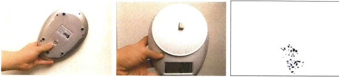
Figure 5-2: An experiment showing that our technique can detect surface tampering caused by very light pressure. To measure pressure, we attach a piece of incompressible rubber to a sensitive scale, shown in (b). We press lightly against the wall with the rubber (a), and zero the scale while touching. The readout from the scale (b) shows that the force is 27 gf. Since surface area of the rubber is 1\text{ cm} \times 1.3\text{ cm} , the pressure is 20.7\text{ gf/cm}^2 . The similarity map relating speckle images before and after touching the wall (c) shows that the touched area can be identified.
