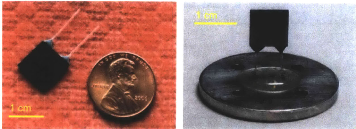
Figure 2. Final assembly of S \mu RE IV [5]. The glass capillaries extend out from the inlet and outlet, allowing the gaseous mixture to flow through the microreactor.
