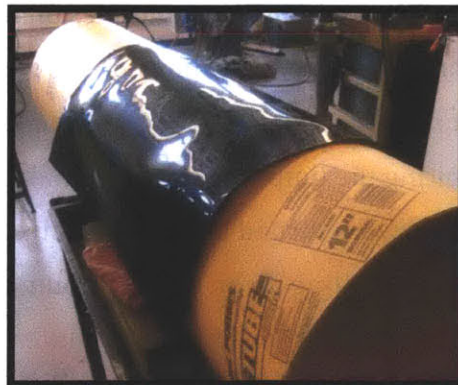
Figure 9: ABS Hood, First Forming Attempt, Photograph
