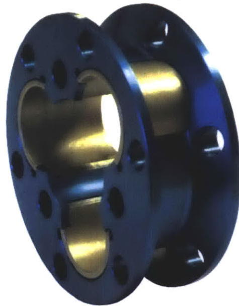
Figure 2.2.3: The Taylor Race Engineering aluminum tripod housing, measuring 84 mm in diameter, 30 mm in width, with a mass of 211 grams, is lightweight and reasonably compact. It is compatible with off-the-shelf tripods, also available through Taylor Race Engineering (8)
