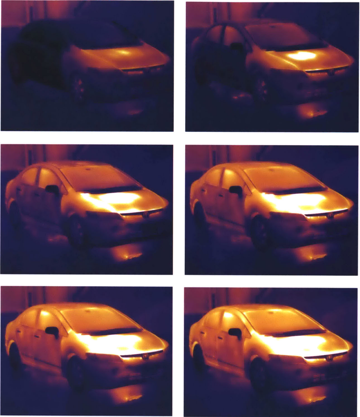
Figure 116: The experiment was to show sequenced thermal images of observed vehicle (2009 Honda Civic) during heating cycle where car heating was turned to the max setting internally, while the external environment was approximately 30 degrees F
