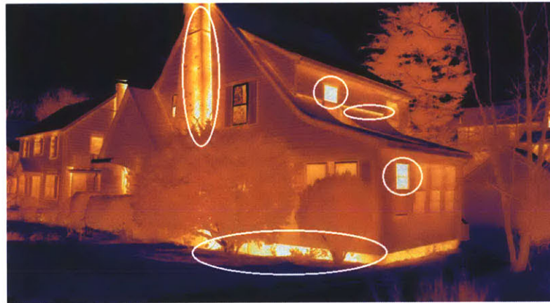
Figure 30: IR image showing high gradient regions that are easy to identify in Home A
