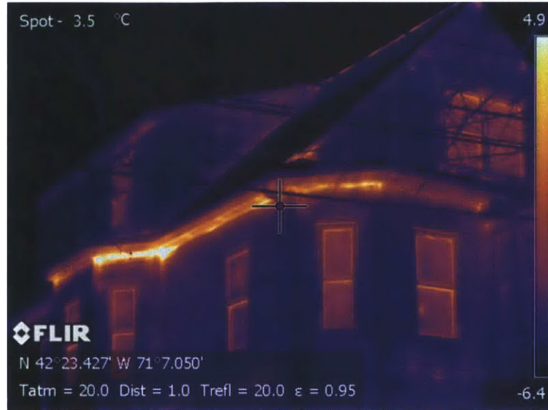
Figure 2: Sample infrared thermal image of home taken with a FLIR LWIR Camera
