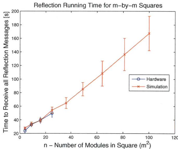
Figure 6-18: The average reflection time in square sheets scales roughly as O(n) , but as explained in Section 6.3.4, this relationship is not guaranteed. The bars on each data point indicate one standard deviation.
