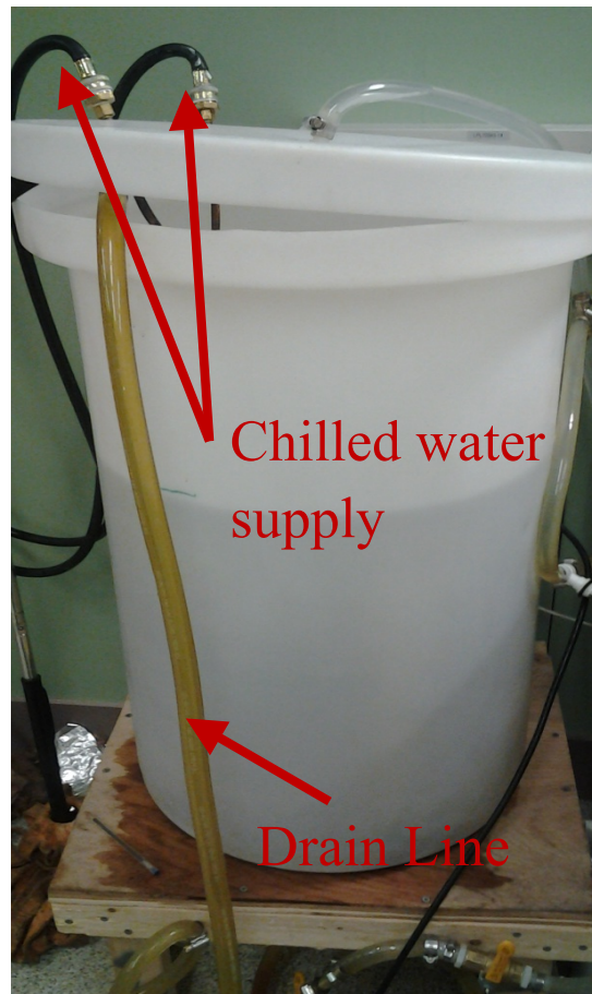
Figure 3-10: Water tank with water supply for the system
