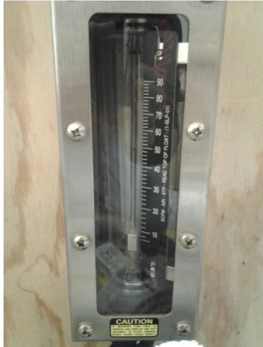
Figure 3-7: Omega in-line air flow meter
