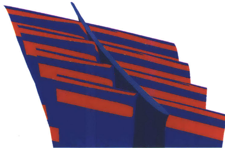
(b) Axial component of vorticity ( \omega_x ) for rotor with 0.2% span tip gap showing negative ( \omega_x ) in tip leakage flow region. Blue is negative (pointing upstream) and red is positive (pointing downstream).
