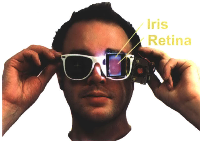
Figure 2-5: We have developed a simple solution that trades complex optics for computation in order to take low quality images and extract the most data from them.
