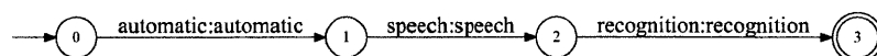
Figure 2-8: An FST that only accepts the word string “automatic speech recognition” and outputs the same word string.
