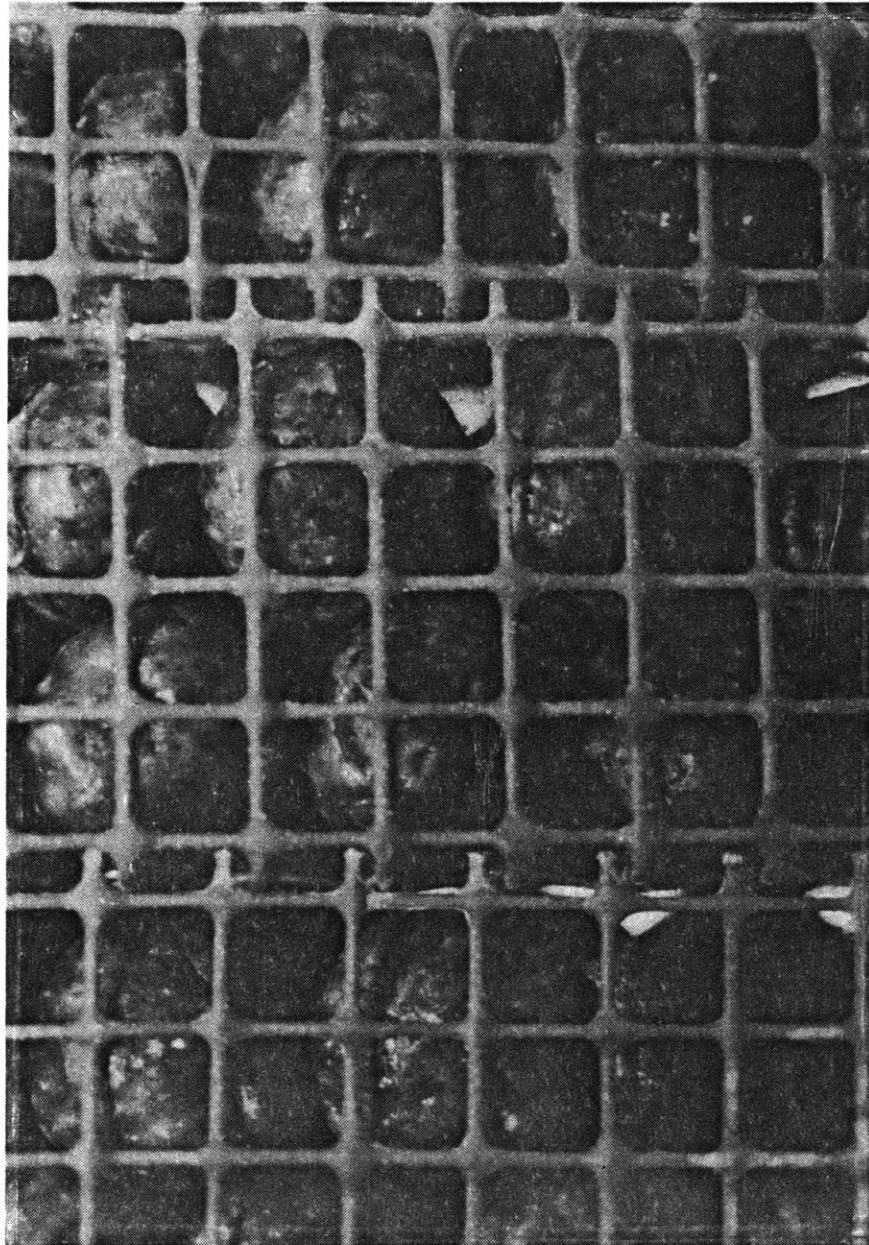
Figure 4.9. Detail of phase-change material after 2 weeks of testing. The white spots on capsules are deposits of salts which have leaked through punctures caused by crystals in the latex coating.
