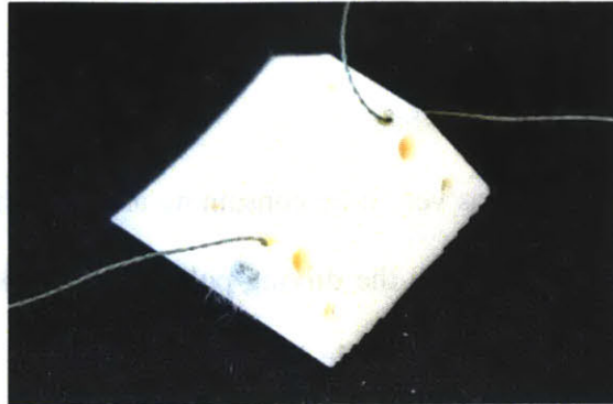
Figure 4-1 Cables are attached to both sides of the top carriage wall with double figure-eight-knot locked in 90 degree holes. The knot is on the vertical wall of the bearing, allowing most of the force of the cable to transmit to the direction of the carriage's motion.
