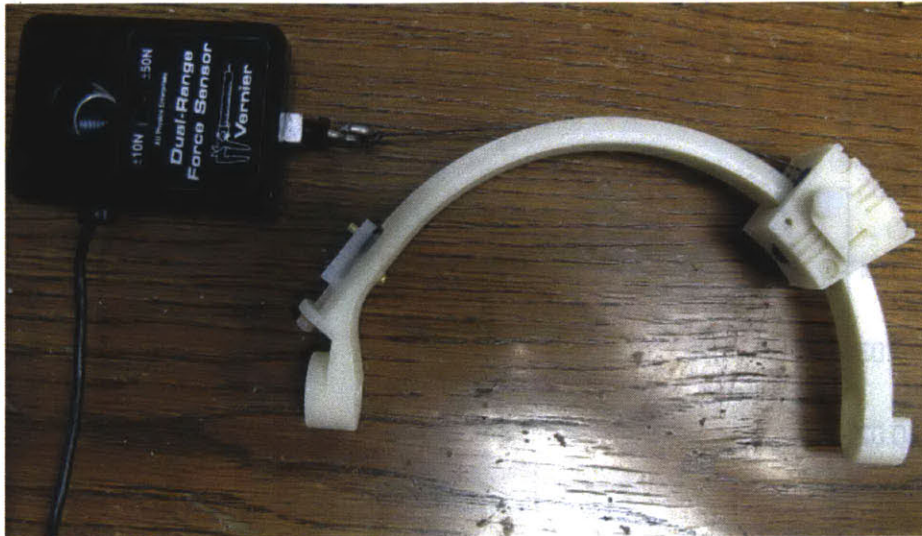
Figure 3-10 Bench level test of the roller bearing with Logger Pro force sensor.
