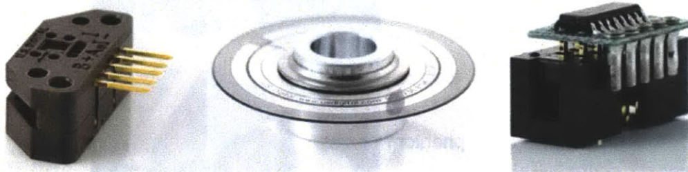
Figure 3-29 Encoder module from US Digital is used with the piezoelectric motor to perform closed loop position control. Left: Optical Encoder module. Middle: 1" diameter encoder disk. Right: Incremental differential encoder cable driver.
