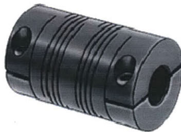
Figure 3-36 Misalignment clamp on coupling is used to connect an extension shaft to the motor shaft [ http://www.mcmaster.com ]. This type of coupling holds onto a shaft with integral clamp and won't damage the shafts like a set screw.
