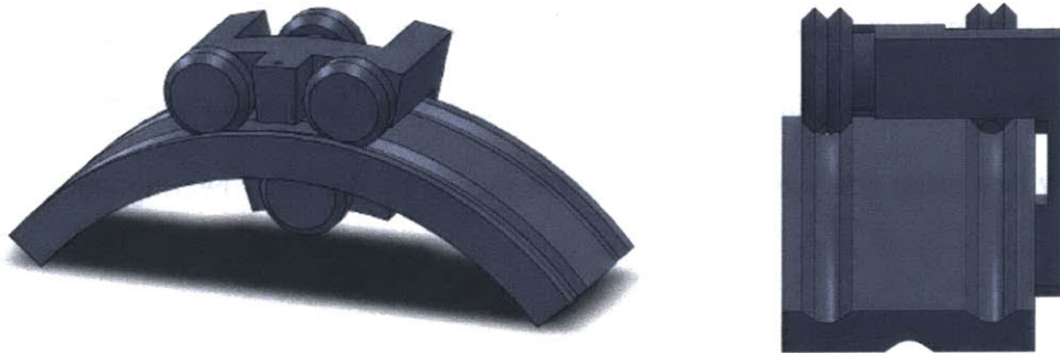
Figure 3-2 Vee groove roller bearing design. Four rollers are required to kinematically constrain the bearing.
