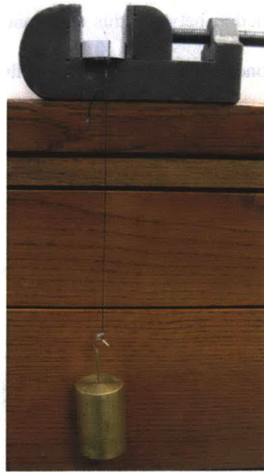
Figure 3-13 Bench level creep test was conducted on Dyneema cable over the course of three days.
