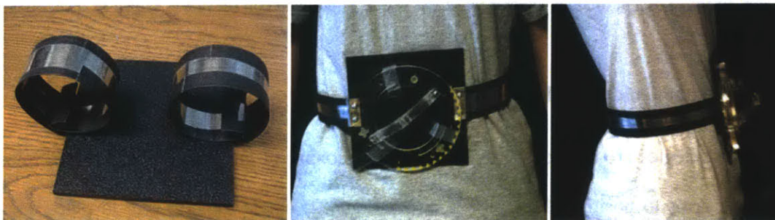
Figure 2-4 Bench level prototype of the device mounting module. Left: The prototype is made of two curved stainless steel bands and a sheet of ABS. Middle: The flexible band naturally wraps around the body and can rigidly support the device (acrylic model). Right: Side view of the prototype.
