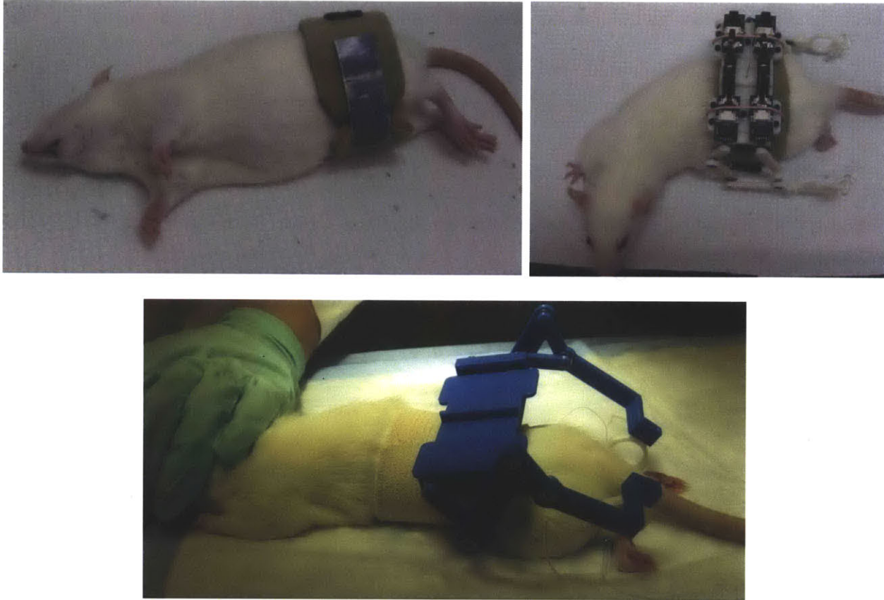
Fig. 4-12. A belt-type harnesses on the animal. (Top-left) the cloth belt was put on the animal while the rat was anesthetized briefly. (Top-right) the rat module was placed on the belt using Velcro tape. This cloth belt easily slipped off the rat's body. (Bottom) the Elastikon® tape around the animal's waist. The tape remained secure on the animal's fur.
