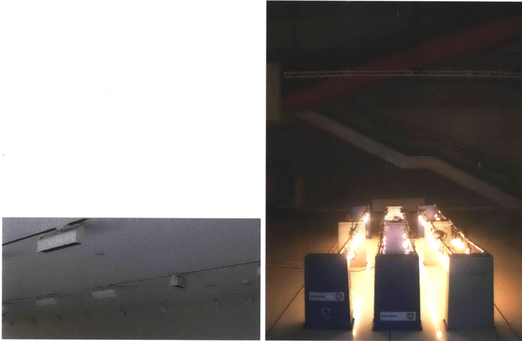
Figure 5-6: (left) Permanent light bank of twenty two 38 W lights installed in the foyer. (right) Temporary light bank of sixty 100 W light bulbs set up in the middle of the atrium.
