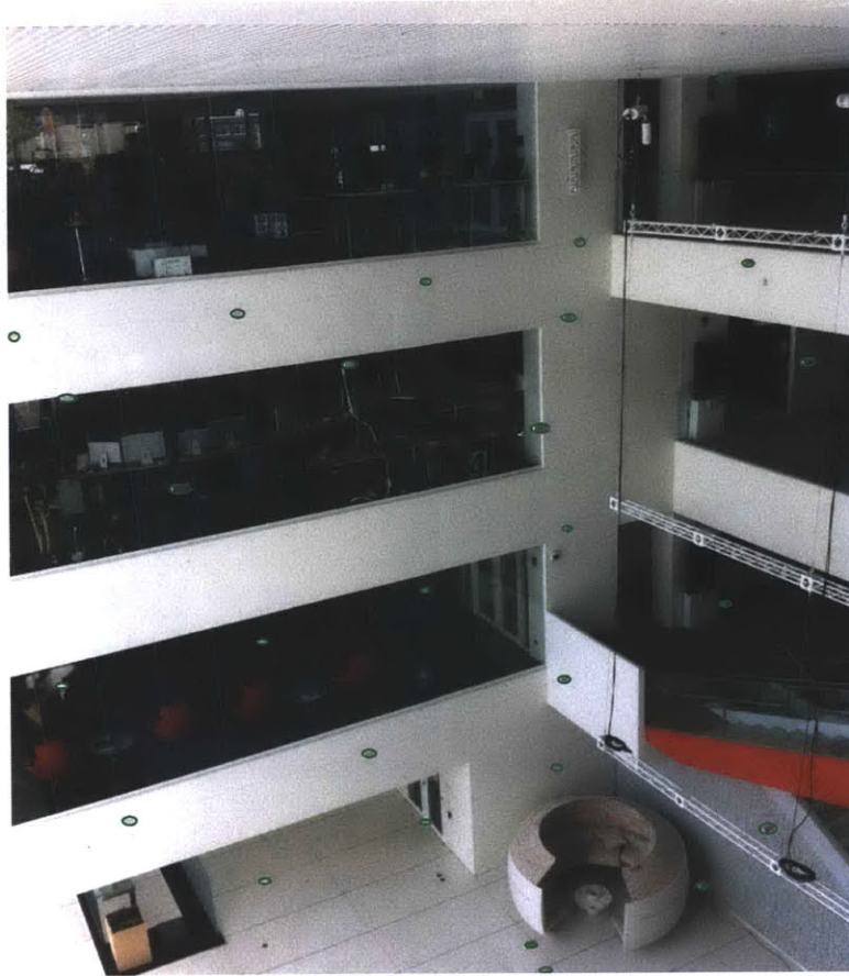
Figure 5-7: Photograph of the atrium with some of the 45 temperature sensors circled in green.
