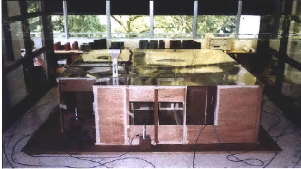
Figure 2-5: Small scale model of an apartment in Singapore used by Wong et al. to investigate the impact of installing a fan in the ventilation chimney [65].
