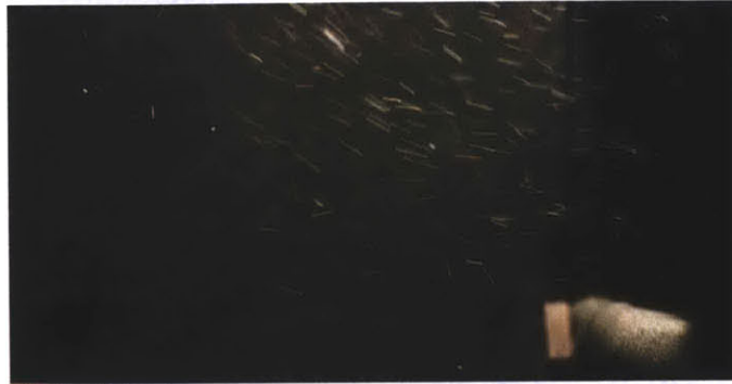
Figure 6-24: Experimental airflow visualization of the entrance from the middle duct into the expanded ventilation shaft.
