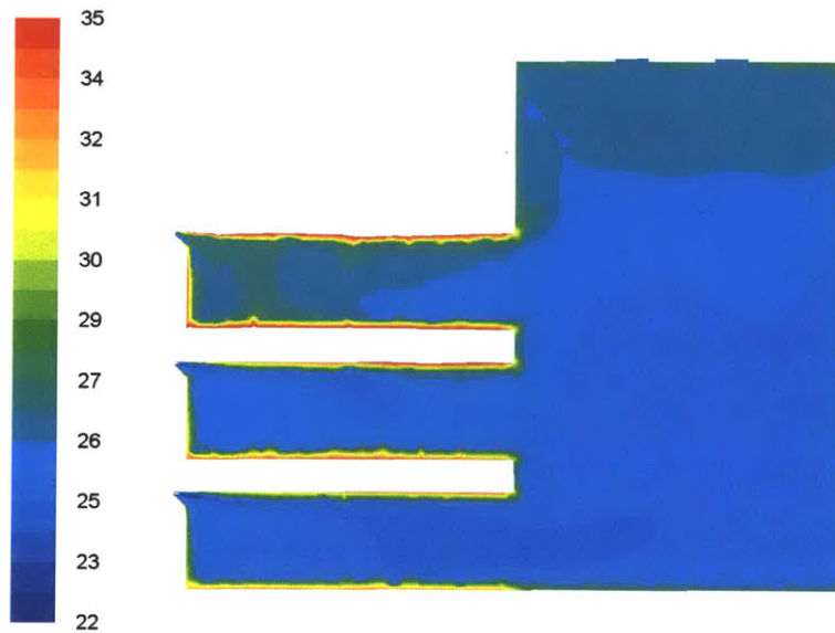
Figure 6-13: Temperature contour in ^{\circ}C taken 6.5 m from the far edge of the 10 m by 10 m atrium in the three story office model. The plane bisects the two nearest exhaust openings in the atrium.
