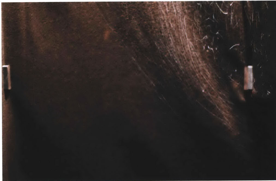
Figure 3-23: Experimental airflow visualization of entrance to model ventilation shaft at the top takeoff duct.
