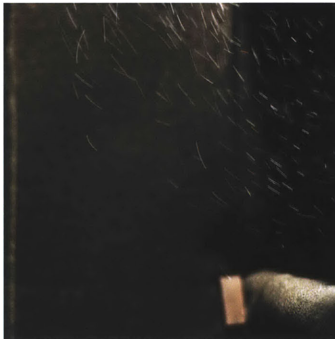
Figure 6-21: Experimental airflow visualization of the entrance from the middle duct into the base case ventilation shaft.
