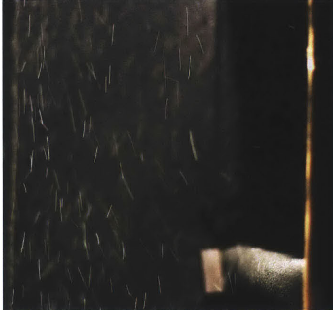
Figure 6-20: Experimental airflow visualization of the entrance from the lower (very bottom of image) and middle duct (large opening on right) into the base case ventilation shaft. Bubbles are introduced at the lower duct.
