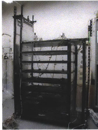
Figure 2-6: Prototype drawing of eight story office building evaluated using a 1:25 scale model, which is also shown. [21]
