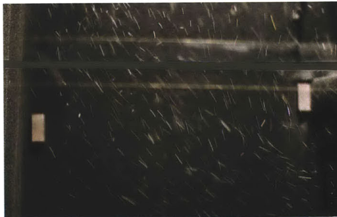
Figure 6-25: Experimental airflow visualization of the entrance from the middle and top duct into the expanded ventilation shaft. Bubbles are introduced into the middle duct. The solid gray line across the entire image is added during post processing to eliminate a bright reflection at the boarder of two acrylic pannels.
