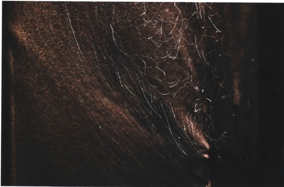
Figure 3-19: Experimental airflow visualization of entrance to model ventilation shaft at the middle takeoff duct.
