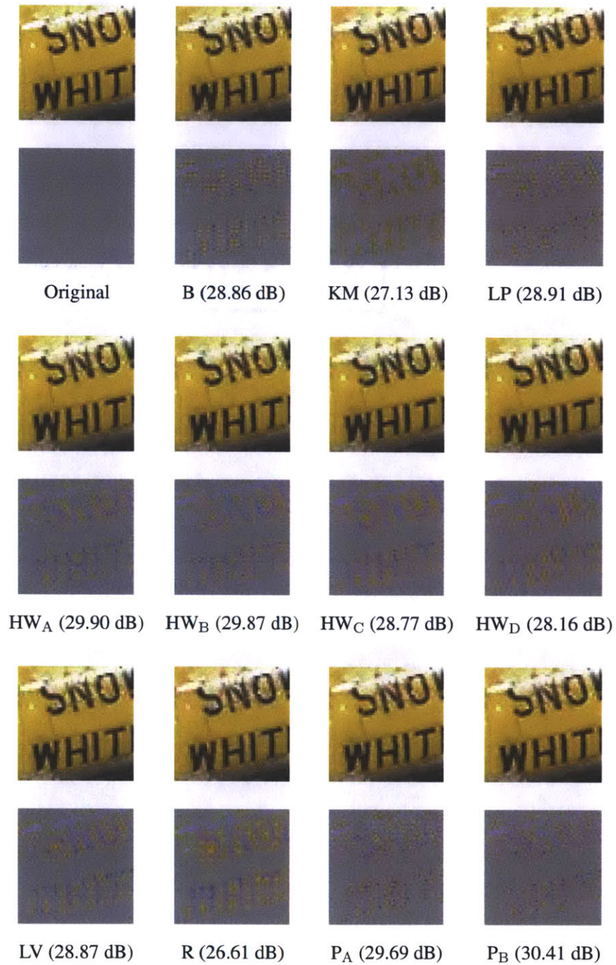
Figure 4.15: Reconstruction and error residual of a selected part from Image 5, for various CFAs. The compared CFAs are Bayer ( B ), Knop & Morf ( KM ), Lukac & Plataniotis ( LP ), Hiraakawa & Wolfe ( HW A –HW D ), Lu & Vetterli ( LV ), random ( R ), and the proposed patterns ( P A , P B ). For recovery, the MoG-based MMSE has been commonly used. Error residual has been measured by reconstruction minus original, with zero displayed in mid-gray. The PSNR score, assessed only on the selected part, is given in parenthesis.
