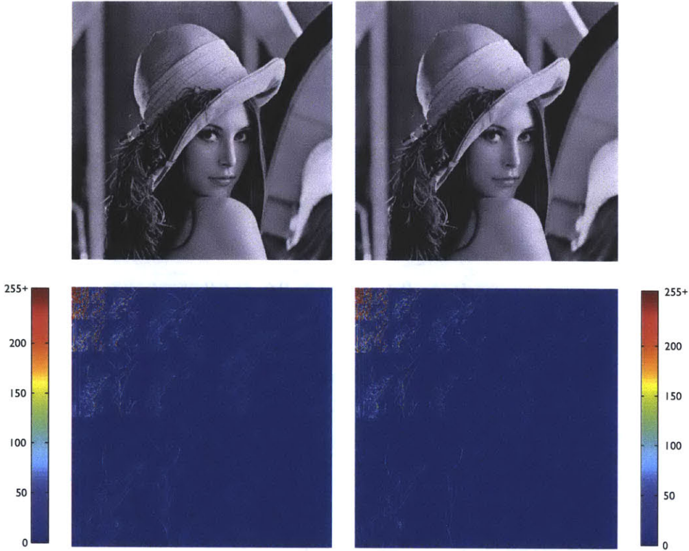
Figure 1.1: Lena images. Left: the original, Right: a sparse approximation. For both, two types of representations are given. Top: pixel-domain, Bottom: wavelet-domain. On the bottom, large magnitudes are represented by warm colors, while small magnitudes are represented by cold colors. The wavelet coefficients of the original Lena show sparsity: most are near to zero. When only the largest 7% of the wavelet coefficients are kept, the resulting image (right) is very faithful to the original (left) whether in wavelet-domain or in pixel-domain.
