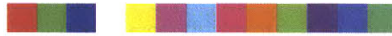
Figure 4.5: Restricted set of color filters: red, green, blue, white (or gray), yellow, magenta, cyan, red+magenta, red+yellow, green+yellow, blue+magenta, blue+cyan, green+cyan. They have been frequently used in the CFA design (see Figure 4.2 for example).
