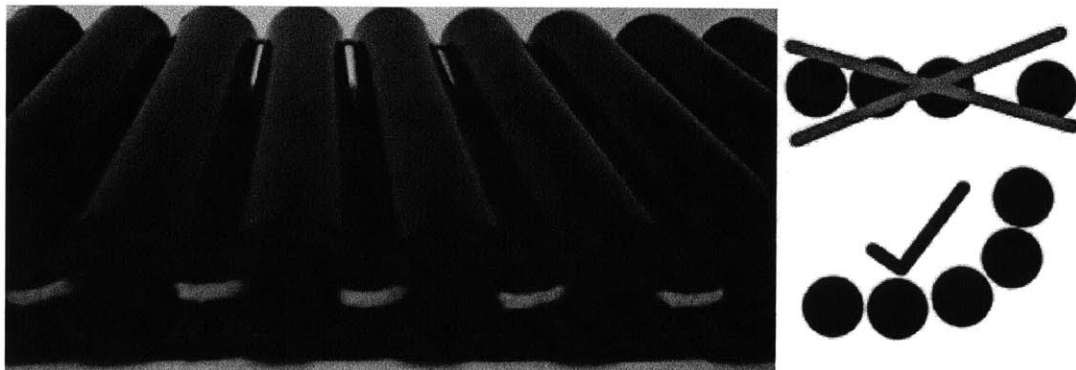
Figure 4-4: The spacers were limited to angular movement.
