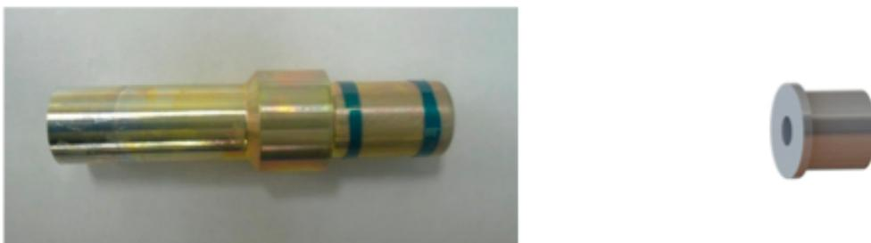
**Figure 4-1: Insert used for experiments (left) and actual A-arm insert (right)**
