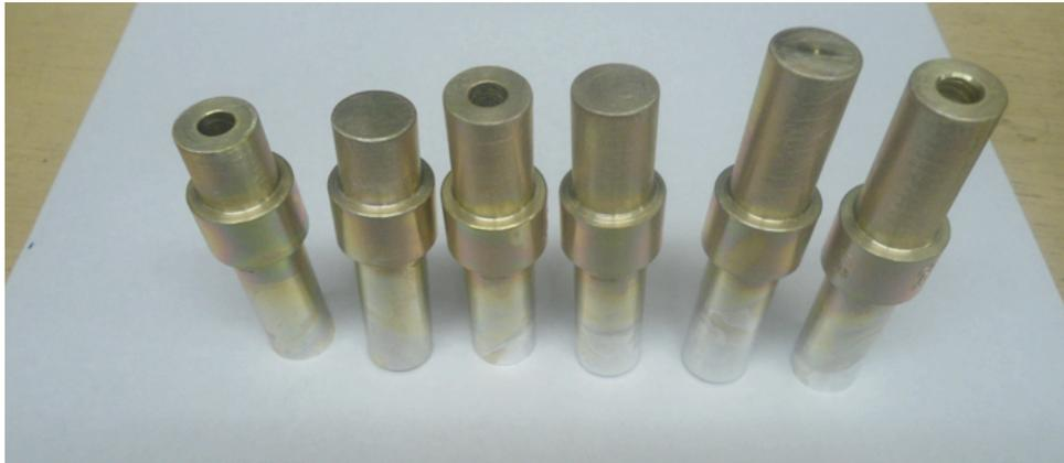
**Figure 5-1: Appearance of aluminum inserts after alodine coating**
