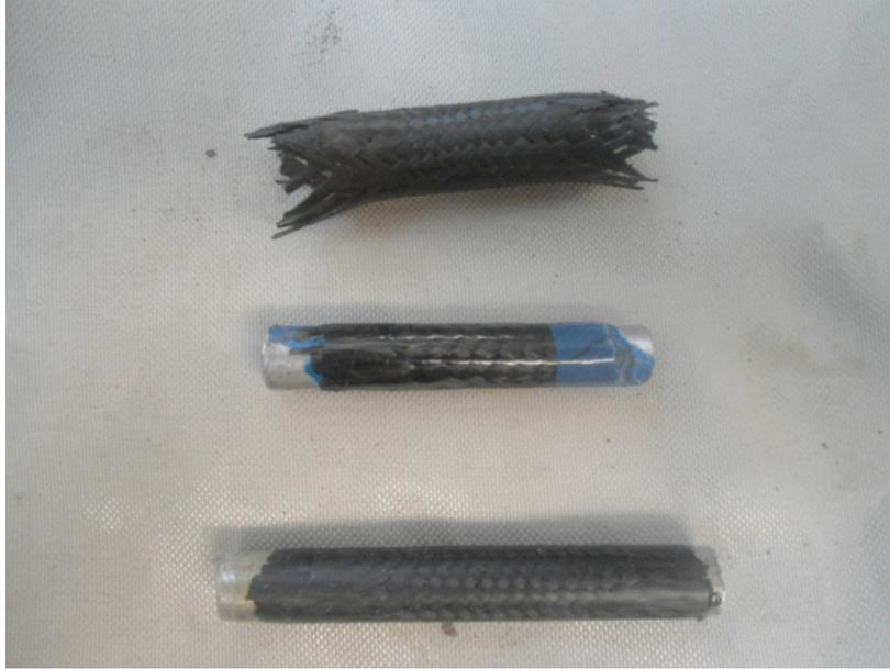
**Figure 5-2: Three methods for laying carbon fiber sleeves**
