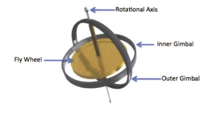
Figure 26: Gyroscope [55]
