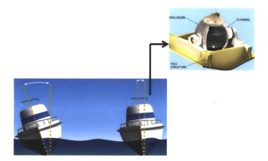
Figure 25: Yacht Motion with (right) and without (left) anti rolling gyroscopes [18,55]
