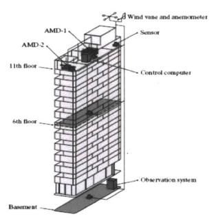
Figure 20: Active Mass Driver System Installation [10]
