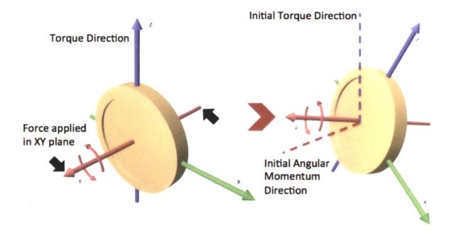
Figure 29: Gyroscope Reaction to Force in XY Plane [55]
