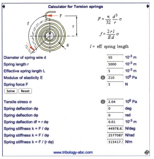
Figure 35: Calculation for Torsional Spring [7]
