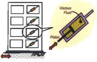
Figure 18: Viscous Damper [13]
