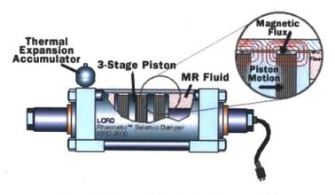
Figure 22: Magneto-Rheological Damper [31]
