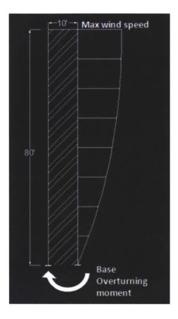
Figure 33: Wind Profile acting on windward side of building
