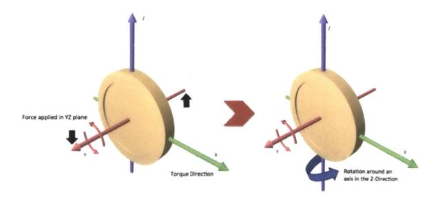
Figure 28: Gyroscope Reaction to force in the YZ plane [55]
