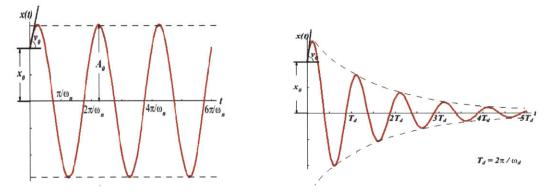
Figure 13: Undamped Response (left) and Damped Response (right) [15]
