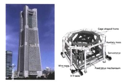
Figure 21: Hybrid Mass Damper in Yokohama Landmark Tower [1]
