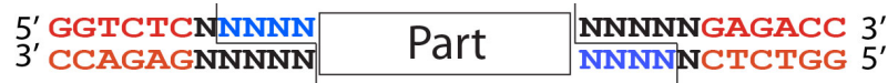
Figure 1. BsaI, a Type IIS restriction enzyme, recognizes a six base pair sequence (red text, 5' GGTCTC 3') and cuts distally at positions +1 and +5. If oriented as shown here, BsaI digestion generates user defined, 5' sticky end overhangs (blue text, N's) flanking the part sequence (Part).
