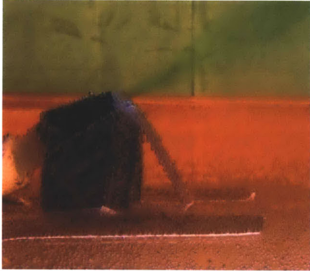
Figure 30. Fully mixed green top layer with orange bottom layer unmixed (picture cropped at surface)
