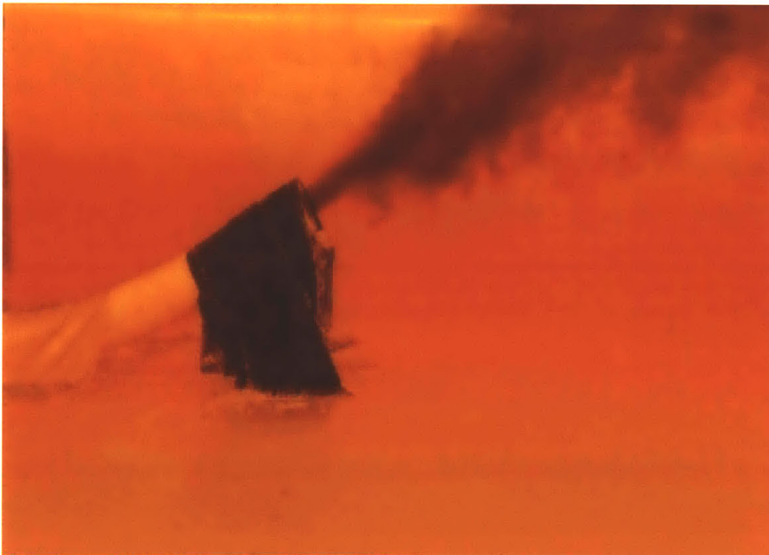
Figure 27. Initial red flow into orange stratification
