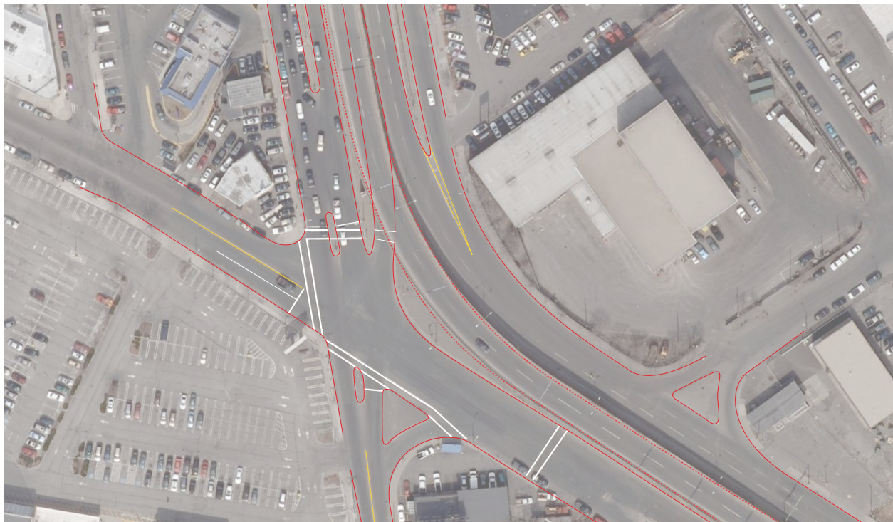
Figure 47: The current configuration of the southbound frontage road and down ramp at Somerville Ave creates a dangerous and confusing weaving movement
